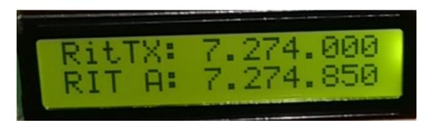
VFO A is in use, and the uBITX will transmit on 7.274.000, and it will receive on 7.274.850
